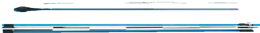
Solar radiation sensors (from top) Dome Net Radiometer NR2 and Tube Solarimeter TSL
